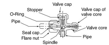
The refrigerant channel is opened so that the refrigerant will flow from the outdoor unit into the indoor unit.
