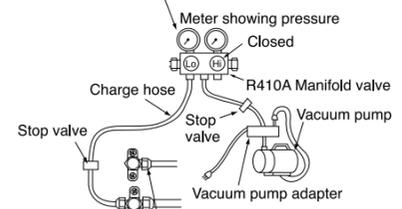
When pumping starts, slightly loosen the flare nut to check of air sucked in. Then tighten the flare nut.
