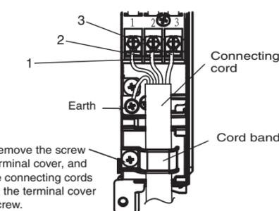
After remove the screw and terminal cover, and put the connecting cords and fix the terminal cover with screw.
